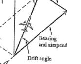
Ex. An airplane with an air speed of 192 mph is flying on a heading of 121°. A north wind is blowing at 15.9 mph. Find the groundspeed and the actual bearing of the plane.
